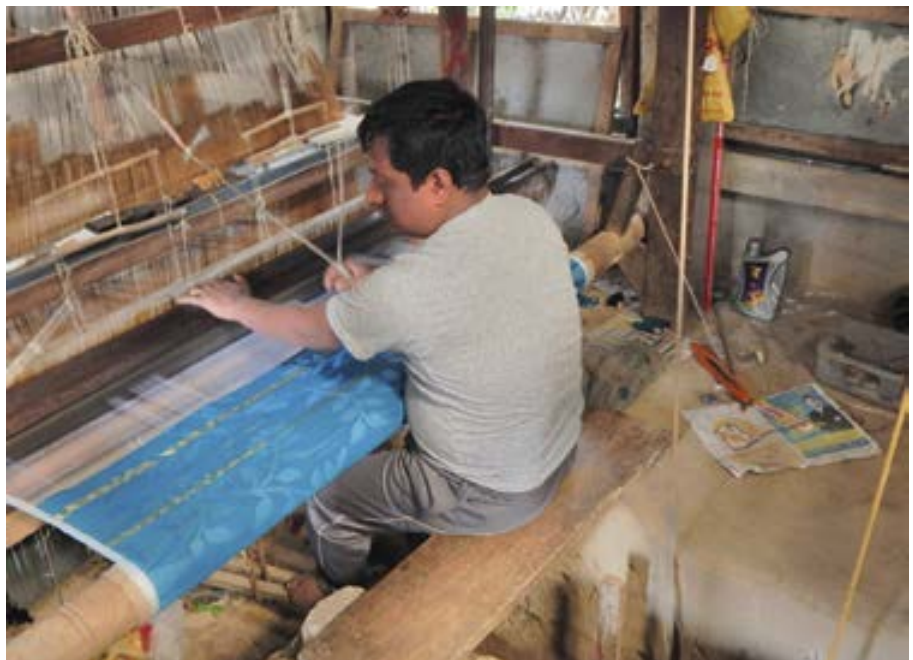
A worker weaving Sari (Traditional cloth worn by Indian women) on a traditional loom
