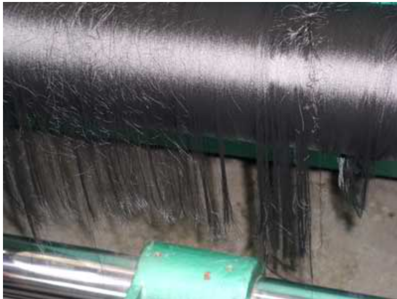
Exhibit 5. A picture of the threads that were being wound on the spool the victim was caught in.
