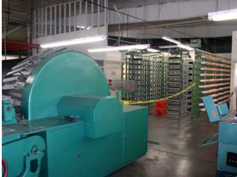
Exhibit 2. A picture of the left side of the machine showing individual spools of thread on racks being fed into it.
