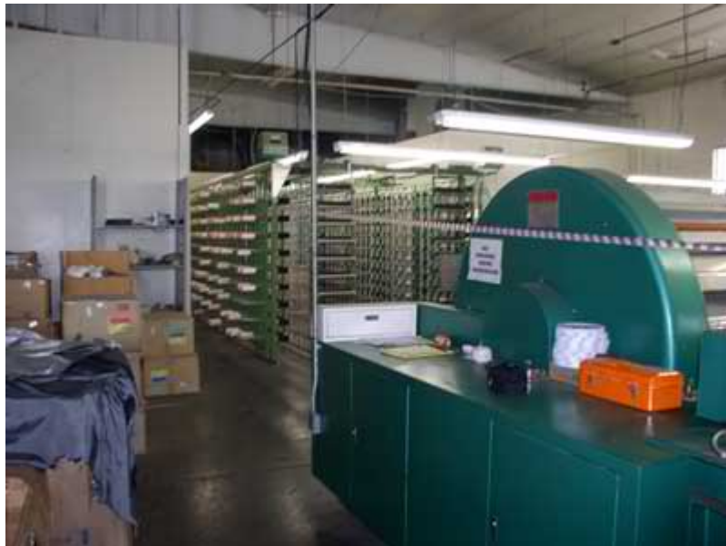
Exhibit 3. A picture of the right side of the machine showing the individual spools of thread on racks that are being fed into it.
