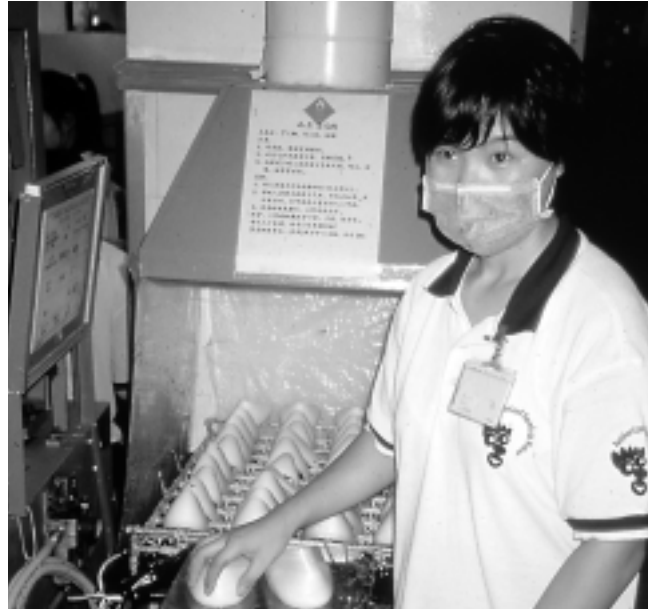
Worker placing shoe parts covered with chemicals in a drying booth in a Dongguan City sports shoe factory. The local exhaust ventilation system had never been tested, as of March 2002, to verify flow rates and capture efficiency. The worker is wearing a "respirator" commonly used in China, which simply consists of a gauze mask with a center section of activated charcoal. This mask does not have an airtight seal and provides no protection to the worker. (Photo by Garrett Brown)
