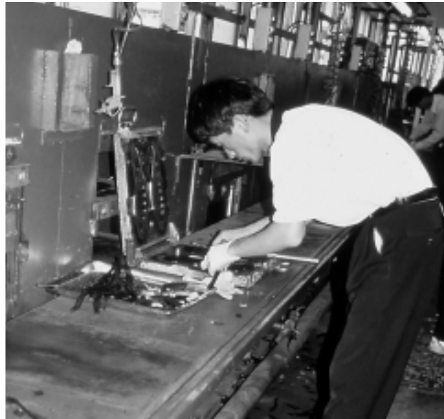
Worker in the "hot press" department of a sports shoe plant in Dongguan City. The workers place shoe sole-shaped pieces of rubber in heavy (15–40 pounds) metal molds which are compressed and heated. Poor design of this work station requires the workers to constantly bend over to place or remove pieces of rubber in the molds. The metal plates are hot and a skin burn hazard, and the molds also pose a foot crush hazard if they fall off the work table. (Photo by Garrett Brown)
