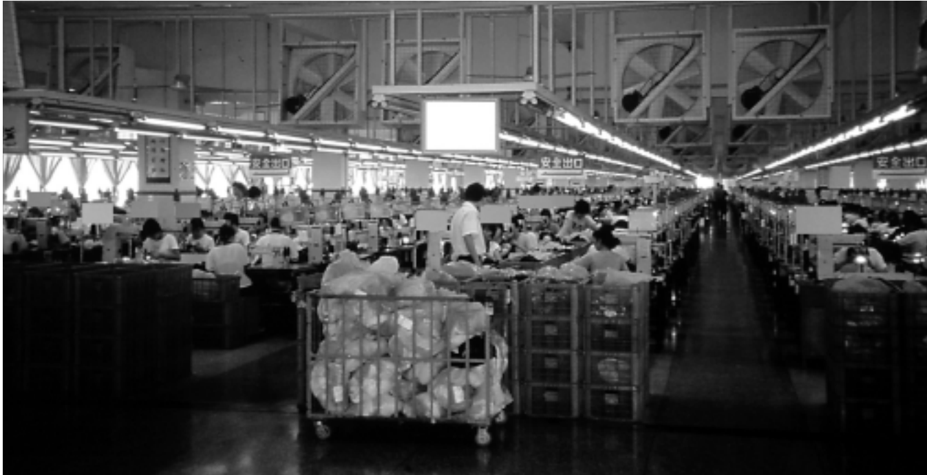
Half of the fifth floor of a sports shoe production building in Dongguan City factory complex with 30,000 workers. In two identical buildings, some 3,000 women workers sit behind sewing machines on the fifth floor assembling the "uppers" of sports shoes to be glued together with the soles of the shoes on other floors of the building. (Photo by Garrett Brown)
