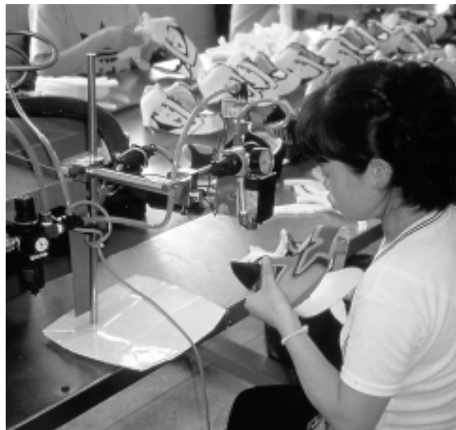
Worker in a sports shoe plant in Dongguan City spraying "hot melt" glue onto shoe parts in preparation for combining cloth parts of the "uppers." This relatively new technology and glue materials create exposures to airborne chemicals that had not been measured or controlled as of March 2002. Several manufacturers of the "hot melt" adhesive do not provide information about the actual components of the mixture so as to "protect proprietary information." (Photo by Garrett Brown)
