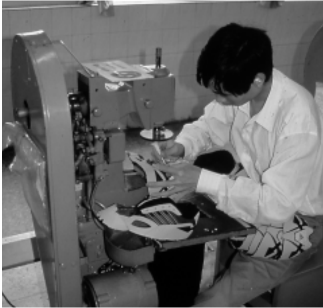
Worker operating a punch press and riveting machine making the holes for shoe laces in sports shoe "uppers" in a Dongguan City plant. The noise levels generated by the machines exceeded 90 decibels (A scale) and required manual placement of metal punches. The workers in this facility used personal hearing protection, but had not received audiograms or training about the hazards of noise-induced hearing loss. (Photo by Garrett Brown)
