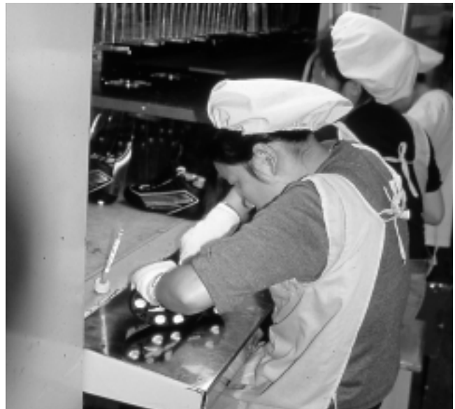
Workers using their thumbs and fingers to insert parts of sports shoes in a Dongguan City plant. Workers are required to elevate their elbows and hunch their shoulders to force parts into place. They also sit on non-adjustable tools without back support. (Photo by Garrett Brown)
