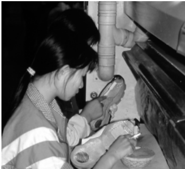
Worker manually applying adhesive to the soles of sports shoes in a Dongguan City factory. The glue is cured by ultraviolet light in the shelves in front of the workers. Hazardous exposures include airborne chemicals, repetitive hand motions, and ultraviolet radiation. As of March 2002, none of the workers had received "hazard communication" training describing the characteristics and hazards of the chemicals they were using or the non-ionizing radiation used to cure the adhesive. (Photo by Garrett Brown)
