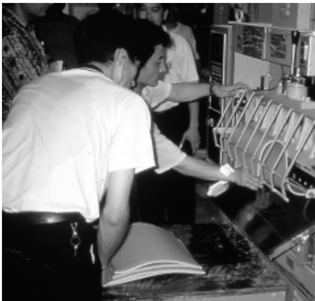
The difficulties of retro-fitting older equipment is evident in this sports shoe plant in Dongguan City. The blue shear cutting polyethylene sheets has been fitted with an orange guard to prevent amputations by the cutting blade. The guard, however, catches the cut materials so workers have to place their hands inside the guard in order to clear jammed polyethylene. (Photo by Garrett Brown)
