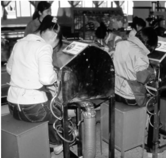
Worker uses a hand-operated buffing tool to clean excessive material from finished sports shoes in a Dongguan City plant. The work is done inside a box intended to capture airborne dust and noise. Noise levels at the operator's station were still above 90 decibels (A scale), however, and other hazards included constant forceful gripping to operate the pneumatic buffing tool and non-adjustable stools without back support. Note the bent necks and hunched shoulders of the workers. (Photo by Garrett Brown)
