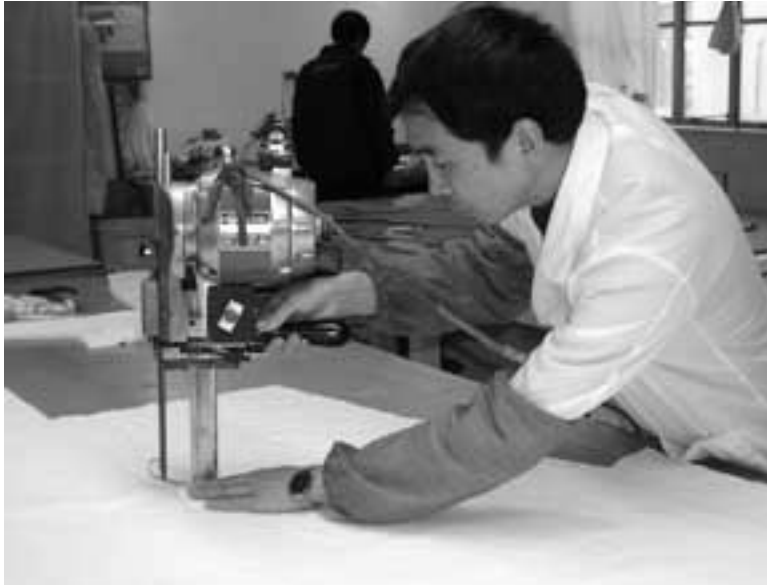
Cutting fabric: a garment factory worker cuts multiple layers of fabric on a cutting table with an electric cutter. This is an example of one of the few men working in this industry. In the textile industry men are usually engaged in maintenance activities, jobs that require heavy lifting, or management.
