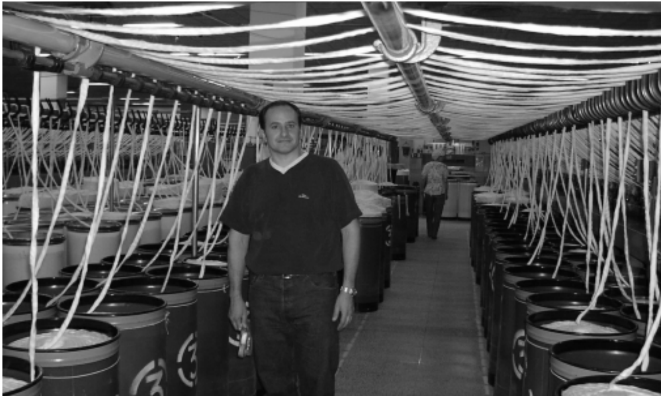
Student in roving: graduate student George Astrakianakis in rows of roving bins. Roving is part of the first stage of cotton thread spinning. Exposures include cotton dust and noise.
