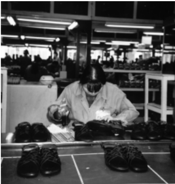
A young Chinese woman applies glue to the soles of sports shoes at a factory in Zhongshan, Guangdong Province, in January 2003. Although factory managers say the workers are instructed to use masks and gloves to guard against fumes and chemicals in the glue, many prefer to work without the protective equipment. (Photo by E. Griggers-Smith)
