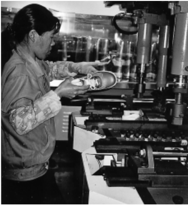
A young Chinese woman operates a machine used to reinforce bonding between uppers and soles at a sports shoe factory in Zhongshan, Guangdong Province, in January 2003. Workers in their late teens and 20s, many from Sichuan and Hunan Provinces, predominate in such factories. Managers say they face intense pressure from their brand-name customers in the West to ensure the assembly line meets labor safety standards. (Photo by E. Griggers-Smith)
